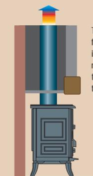
There is also a top flue outlet for installations that require the flue pipe to travel from the top of the stove.
