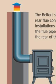
The Belfort standard has a rear flue connection for installations that require the flue pipe to exit from the rear of the stove.
